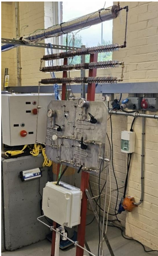
Figure 4: Picture of the test rig showing the heating section, the cooling bundle and the control/measurement devices.
