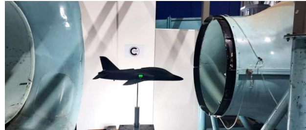
Figure 2: Passive test of a 4-DOF BAe Hawk model in wind tunnel
