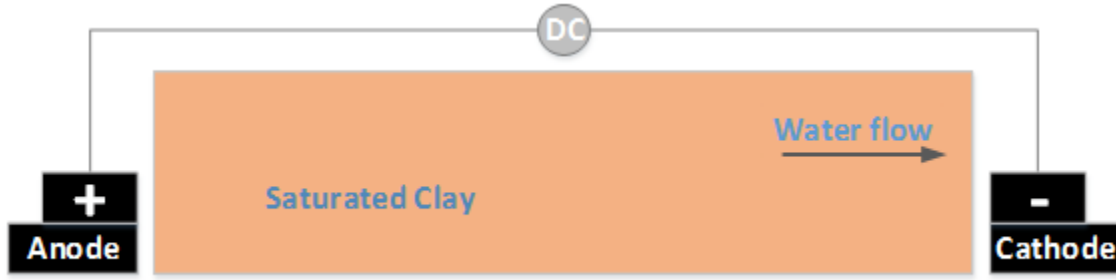
Fig. 1 Electro-kinetic phenomena: electro-osmosis (adapted from [8])
