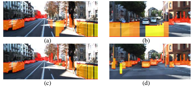
Fig 5. (a),(b) stixel estimation using original algorithm (c),(d) stixel estimation using the extended algorithm (best seen in color)
