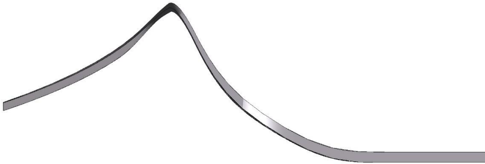
Figure 6. Geometric configuration of liquid oxygen additively manufactured (AM) cooling channel of the DemoP1 aerospike engine demonstrator developed by Pangea Aerospace.
