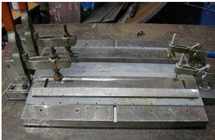
Fig. 2 Clamping arrangement for plates.
