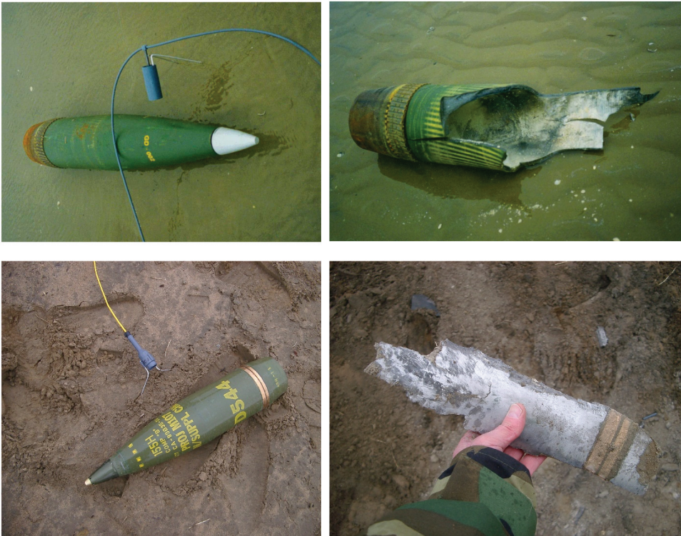
Figure 4. (A-b) typical low-order of a British 155 mm projectile (c-d) a violent low-order of an American 155 mm projectile resulting in smaller fragments photos Alford Technologies Ltd.
