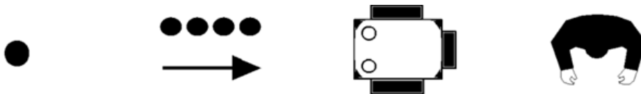
Figure 1: Basic elements in DES (from left to right: a part, a buffer, a machine and labour).
