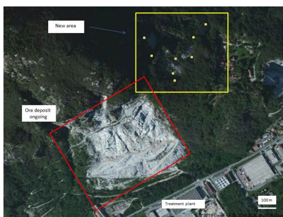
Figure 4.a: Location of the samples in the new investigated area. The dot points represent the samples location
