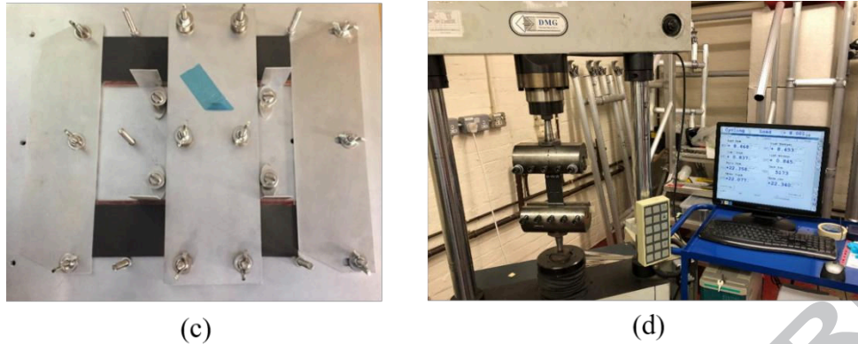
Figure 2: Wide lap joint used in this study: (a) side view, (b) top view showing a semi-circular initial disbond; geometry and dimensions are adopted from [9] (unit: mm). Fatigue cracks were monitored from the four corners of the adhesive bond, marked as A, B, C, D. (c) clamping plates with fasteners to ensure uniform adhesive thickness, (d) fatigue experiment setup
