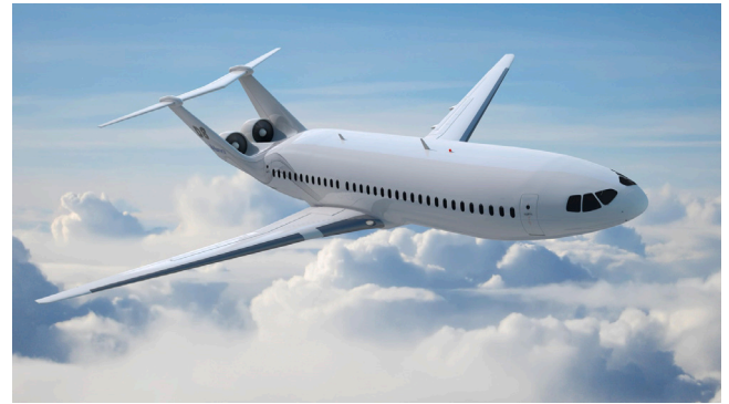
Fig. 2. Render of the D8 “Double Bubble” aircraft concept.
