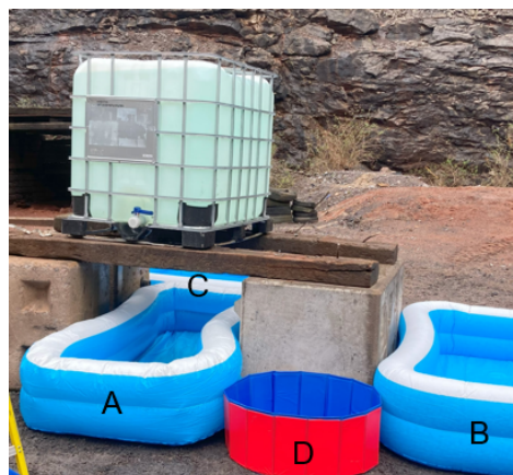
Figure 1: Experimental set up at Alford's range showing all four paddling pools A, B, C and D as well as the IBC filled with 1000 L of water suspended on top of two solid wood beams.
