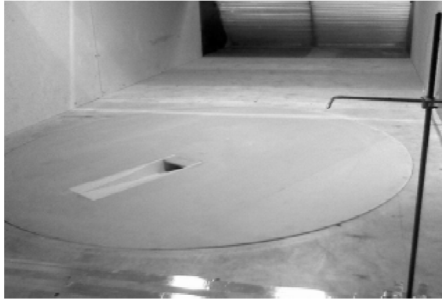
Figure 2a. View, looking downwind, of the ABLWT working section with the NACA intake mounted in the adjustable turntable
