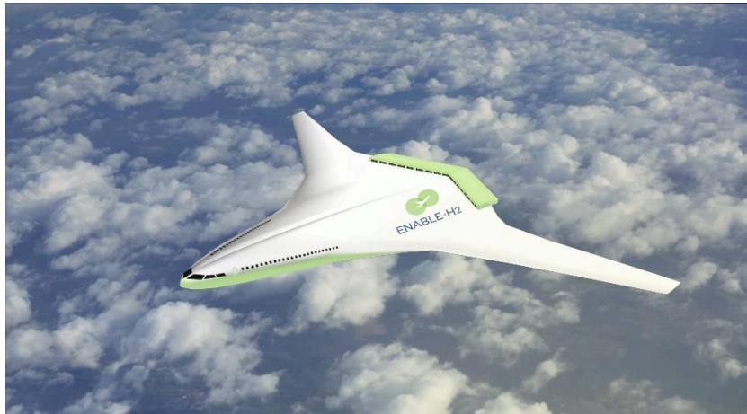
Figure 14- rendition of LR- max synergy concept BWB aircraft.
