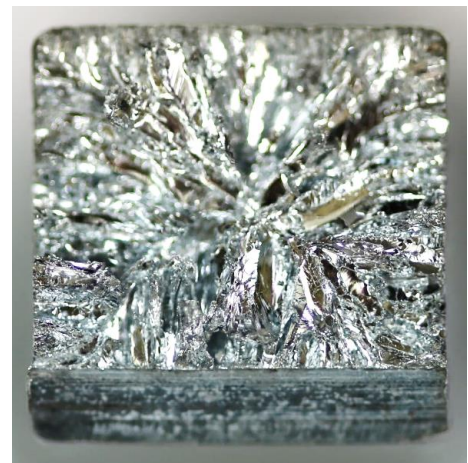
Figure 5 - Zinc Fracture Surface
