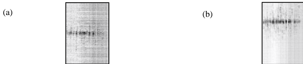
Figure 7. OCT mages obtained from a mirror surface (inverted greyscale) accumulating (a) 1 and (b) 10 frames for each phase range.
