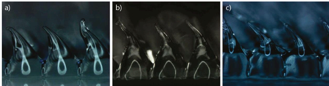
Figure 14: Optical microscopy images of asymmetric pyramid shaped PDMS created by selective disengagement at different angles where a) 35\pm 1^\circ b) 44\pm 5^\circ and c) 50\pm 1^\circ [170]
