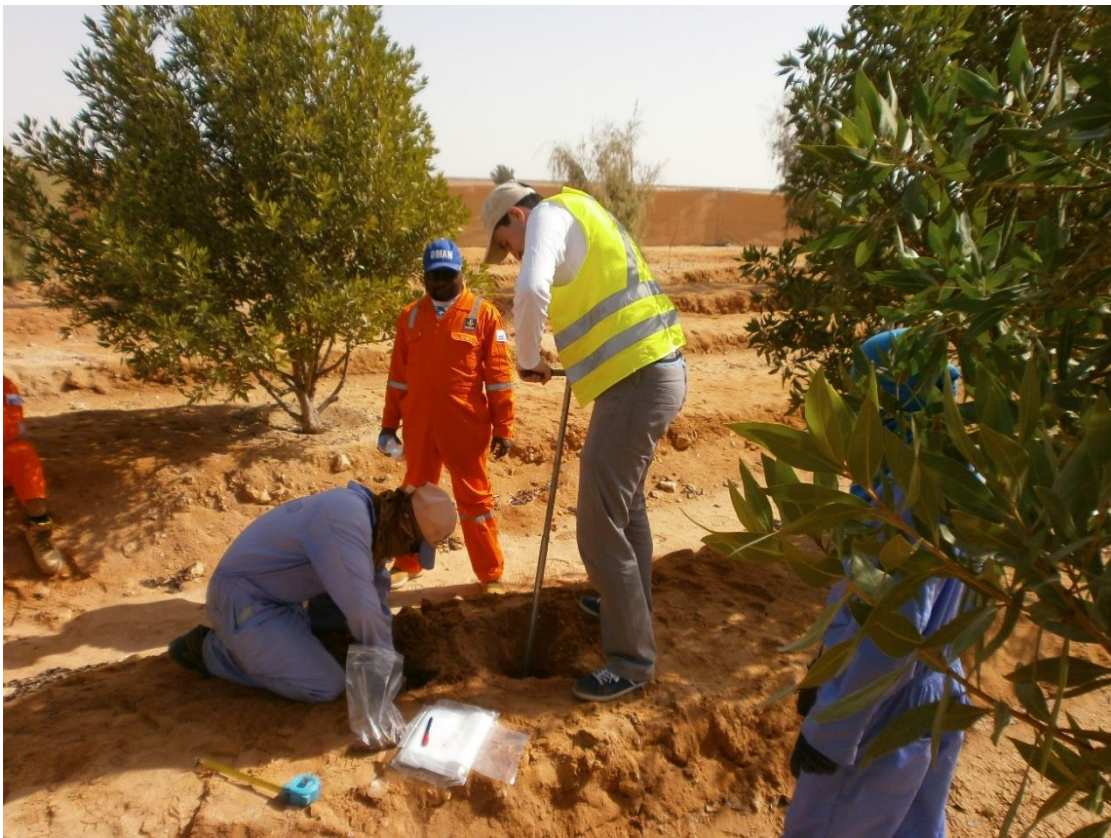
Sampling of disturbed soil at 25 cm and 50 cm of depth.
