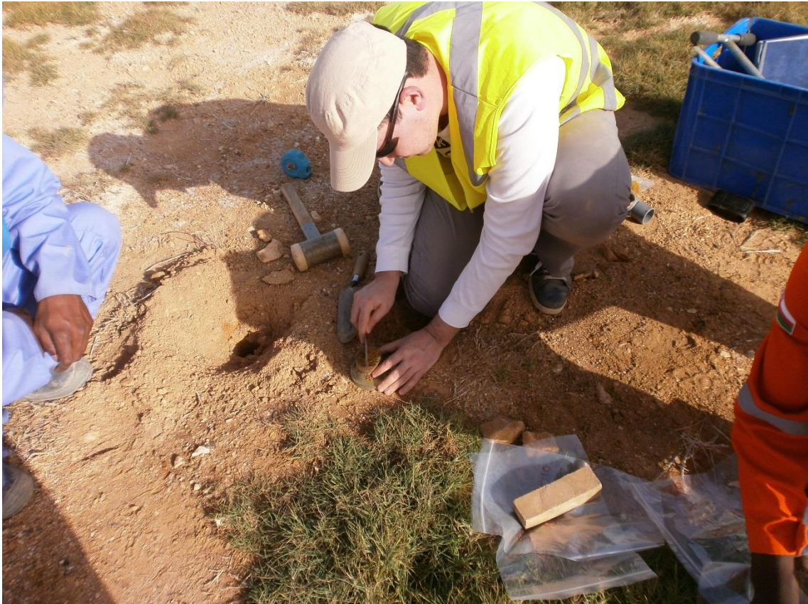
Sampling of disturbed soil 25 cm of depth for bulk density measurement.
