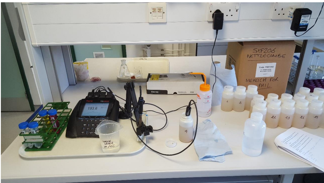
Measurement of the electrical conductivity at 25°C of soil samples diluted in water for the determination of the soil gypsum content with a conductivity meter (Orion™ Versa Star Pro™, ThermoFisher).
