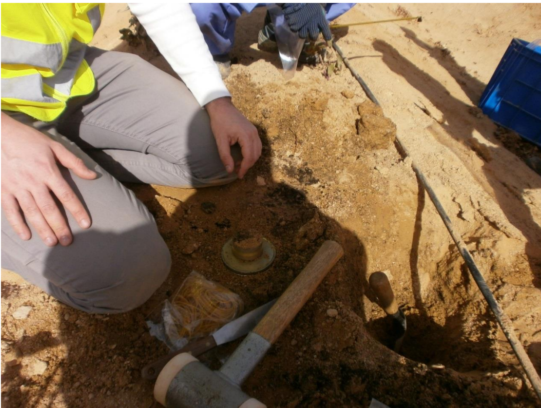
Sampling of undisturbed soil at 25 cm and 50 cm of depth.
