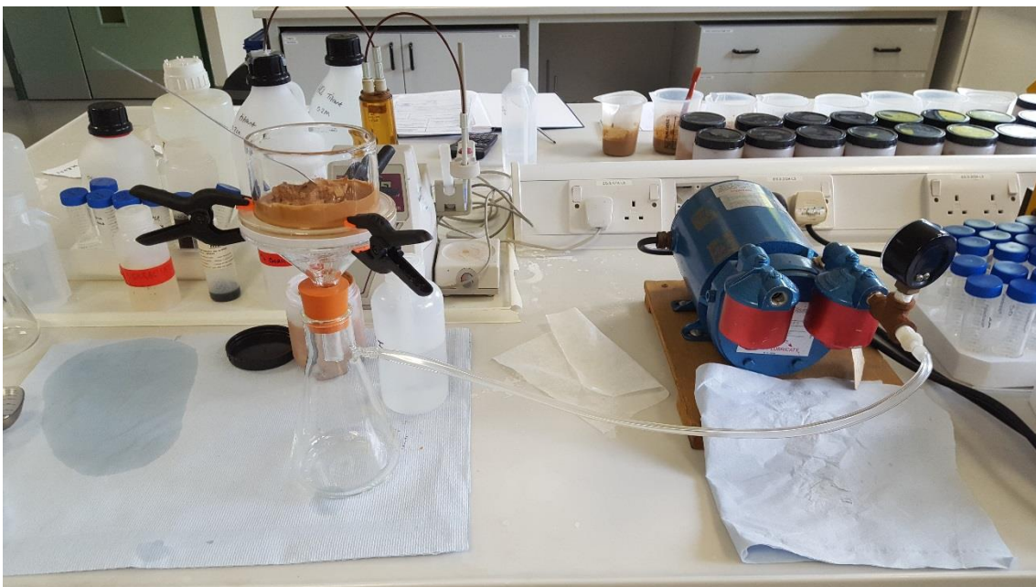
Extraction of the soil saturation extracts.
