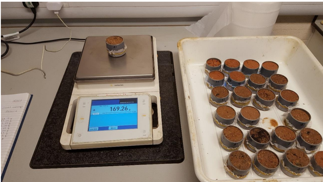
Water-saturated undisturbed soil samples being weighed.
