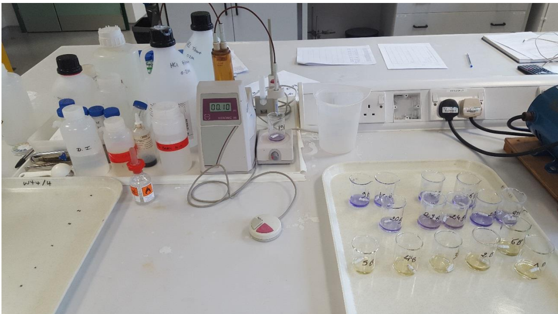
Measurement of the alkalinity (as \text{CaCO}_3 equivalent) of the soil saturation extracts with an automatic titrator (TITRONIC® 96, SCHOTT).
