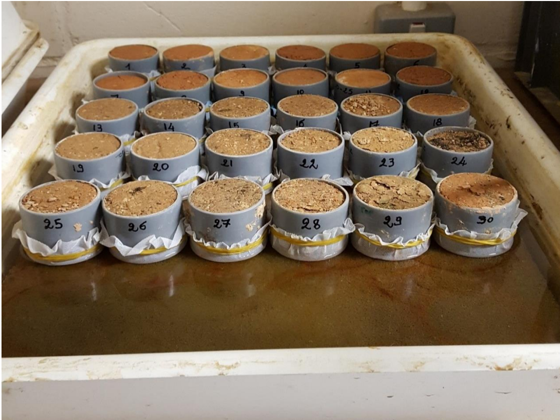
Undisturbed soil samples being water-saturated on foam wetting-up bath.
