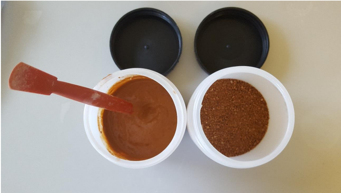
Preparation of a saturated soil paste (left) from air-dried soil (right).
