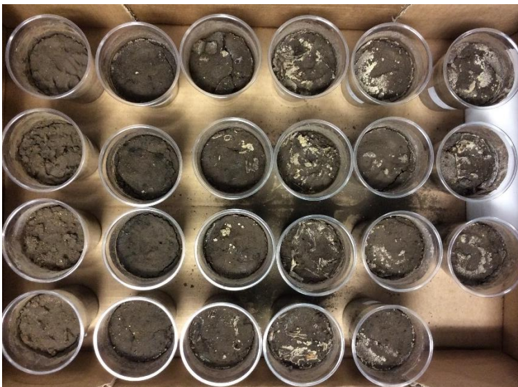
Photo 3-1 Pots at 14 (top left), 30 (top right) and 90 (bottom left) days after treatment application. Treatment order from left to right in each photo is: Soil only, LD + biochar, LD + woodchip, LD + Straw, LD + Glycerol and Liquid Digestate (LD). Pots were lined up by treatment for photo then returned to positions according to randomised block design.
