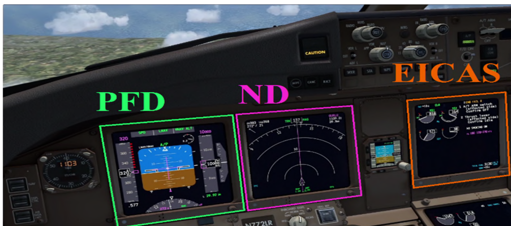
Figure 2. The analysis of visual parameters shifting among PFD, ND and EICAS on the flight deck
