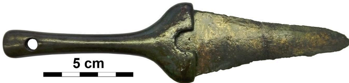
Figure 1 – Bronze Age dagger from Koban, Republic of North Ossetia-Alania, Russia. The color of the hilt was silverish while the blade had a warm, golden-like color. The hilt contains about 9.8 wt.% arsenic and no tin, while the blade contains 10.1 wt.% tin, and no arsenic. Today, the dagger is very much corroded, so the original colors of the metals are no longer visible (Photograph: M. Mödinger, © Naturhistorisches Museum color).
