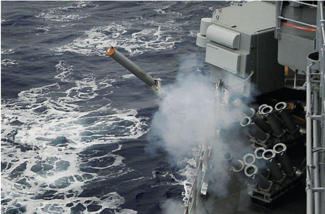
Figure 1-18: A Mark 36 Super Rapid Bloom Offboard Countermeasures (SRBOC) device launching its offboard decoy from the deck of the Ticonderoga-class cruiser USS Lake Champlain. (Image sourced from [73].)
