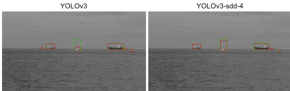
Figure 6-12: Bounding boxes predictions (drawn in red) from YOLOv3 and YOLOv3-sdd-4 and ground truth labels (drawn in green) for a frame of near-infrared test data.
