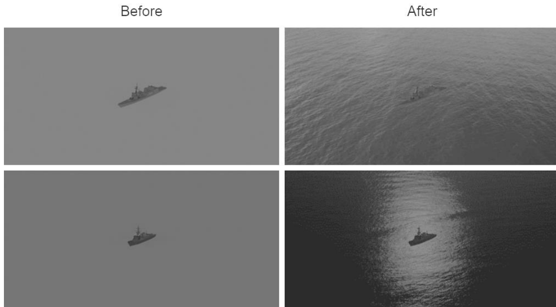
Figure 3-18: Sea-state augmentation of synthetic infrared images where the sea-sky horizon line is not visible. (Image brightness and contrasts have been enhanced for illustrative purposes.)
