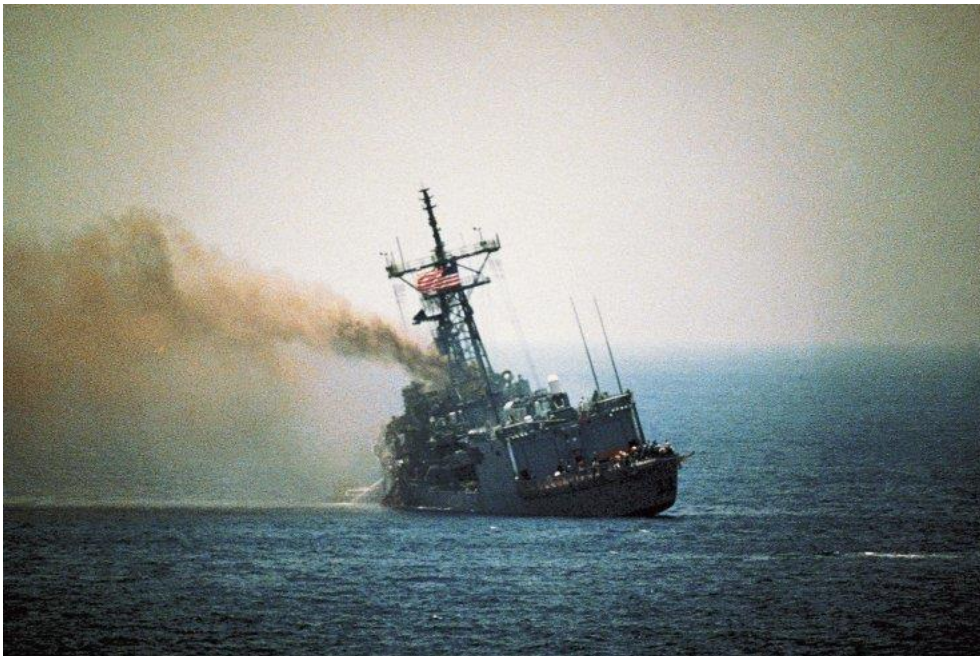
Figure 1-25: An image of the serious damage caused to USS Stark after being hit by an air-launched Exocet anti-ship missile during operations in the Arabian Gulf in May 1987. (Image sourced from [73].)
