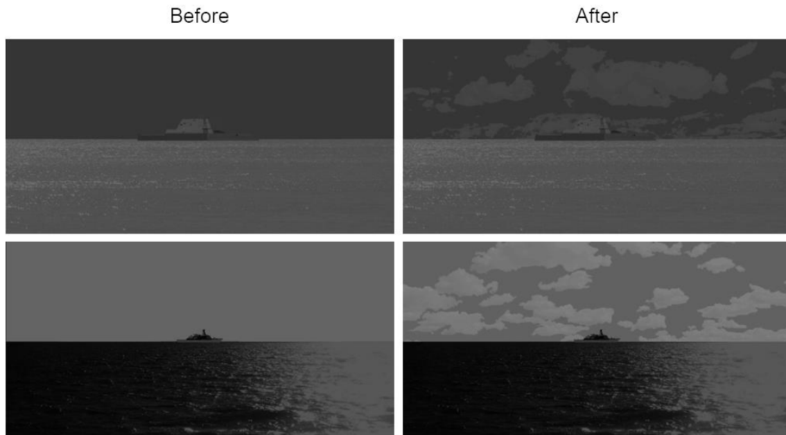
Figure 3-20: Sky-state augmentation of synthetic infrared images. (Image brightness and contrasts have been enhanced for illustrative purposes.)
