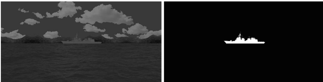
Figure 5-11: An example of an augmented synthetic input image (left) and its corresponding binary label image (right).
