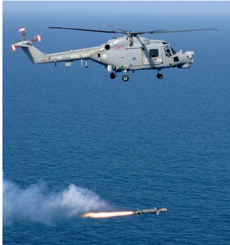
Figure 1-1: Launch of a Sea Skua lightweight anti-ship missile from a Westland Lynx helicopter during a two-week trial period at the Aberporth Range, UK in 2006. (Image sourced from [14].)
