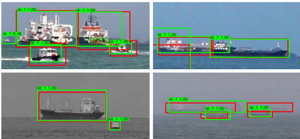
Figure 2-2: A selection of images from the evaluation of Mask R-CNN with predicted and ground truth boxes drawn in green and red respectively. (Images sourced from [125].)
