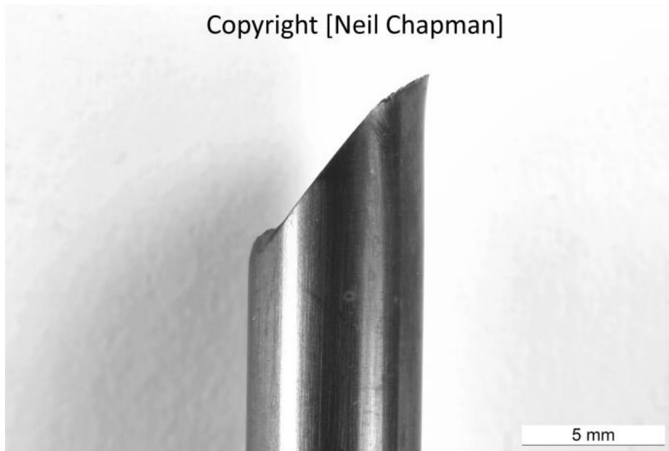
Figure 6.4: Low powered optical microscope image of fractured test specimen showing the typical 55° crack/fracture angle produced from fatigue testing in air using the 10-1-1-1 s waveform and non-precorroded test specimen
