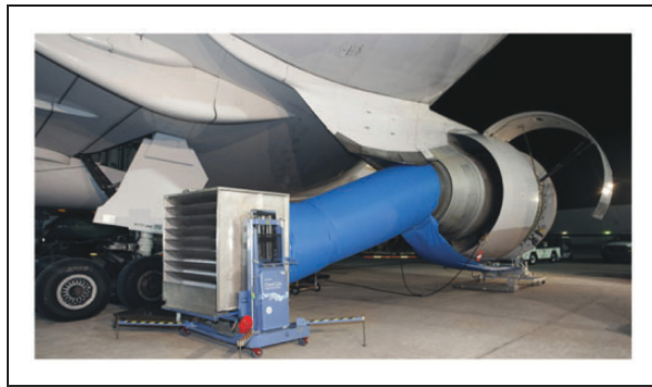
Figure 4. On-wing compressor washing with capture of effluents. 8
