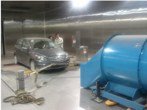
Fig. 2. The testing vehicle with a chassis dynamometer during experiments.
