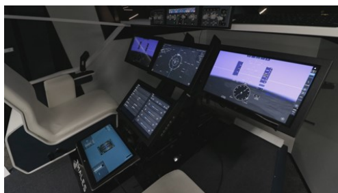
Fig. 2. Thales future cockpit simulator.
