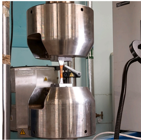
Fig. 4. Illustration of the fatigue testing using a 100 kN servo-hydraulic machine.
