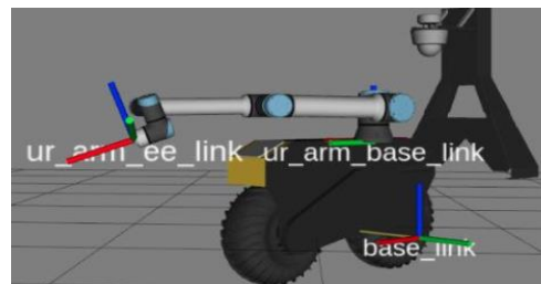
Fig. 3. Transformation between two coordinate frames
