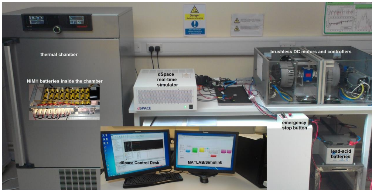
Figure 1: Battery HIL test rig and its components
