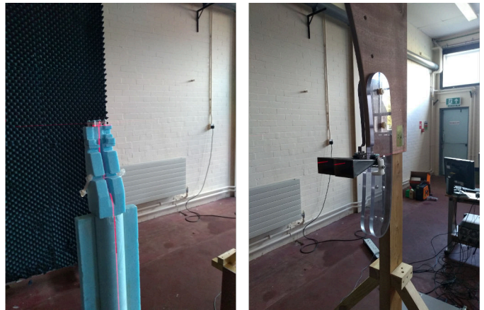
Fig. 2. Photo of the aligned setup showing the laser vertical and horizontal lines on the target and horns.
