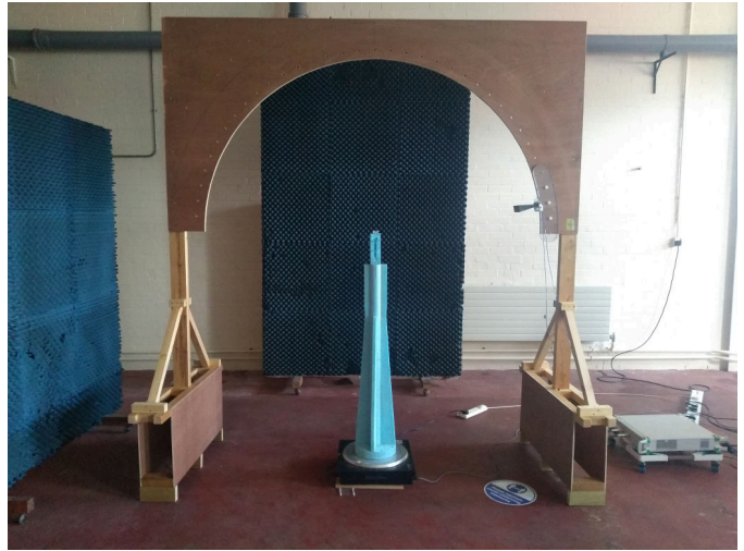
Fig. 1. Photo of the setup with horns pointing the drone from an aspect angle of 10 degrees in elevation.
