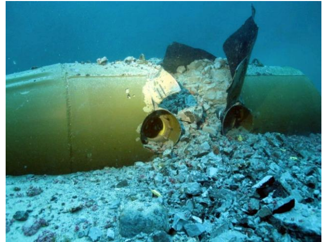
Partial low-order on a thin-skinned mine shows that a larger charge was needed to cause pressure to build up within the entire mine before bursting. (Image courtesy of Royal Norwegian Navy)
