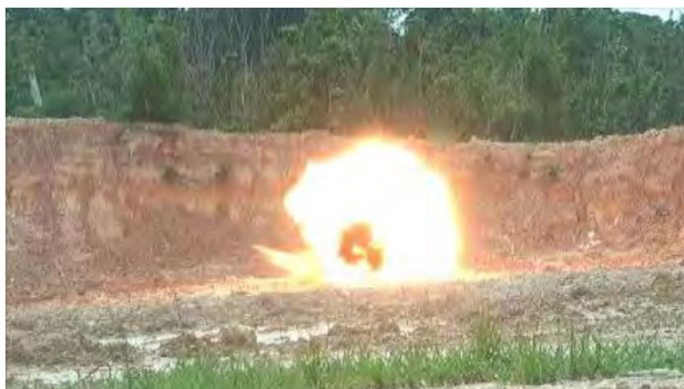
Fig. 6. Typical fireball from low-order of a 1000lb Mk 82 bomb
