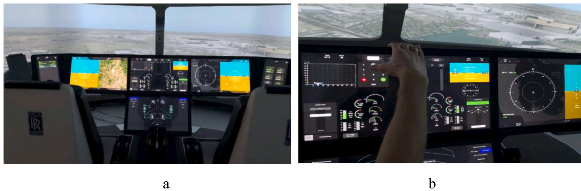
Fig. 1. Future Systems Simulator (FSS) (1a) is a highly reconfigurable modular flight simulator with repositionable seats, displays, sidestick pedestals, thrust levers and touchscreen monitors, which are used as control inputs. The touchscreen monitors can be fully modified to satisfy the needs of the research (1 b).
