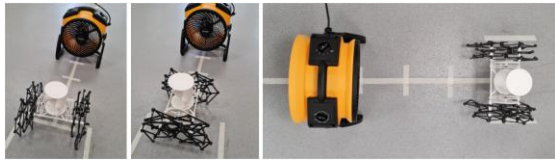
Figure 8 Experimental set-up for integrated robot testing
