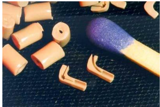
Figure 4: Micro cochlear implants, compared with the head of a safety match (courtesy of Battenfeld).
