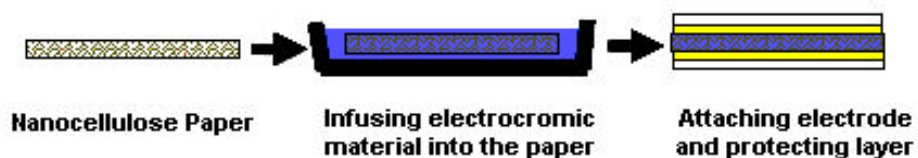
Fig. 18 Fabrication process of the display using nanocellulose
