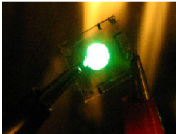
Fig. 20 Cellulose Nanocomposite based Flexible Organic Light Emitting Diode (FOLED)
