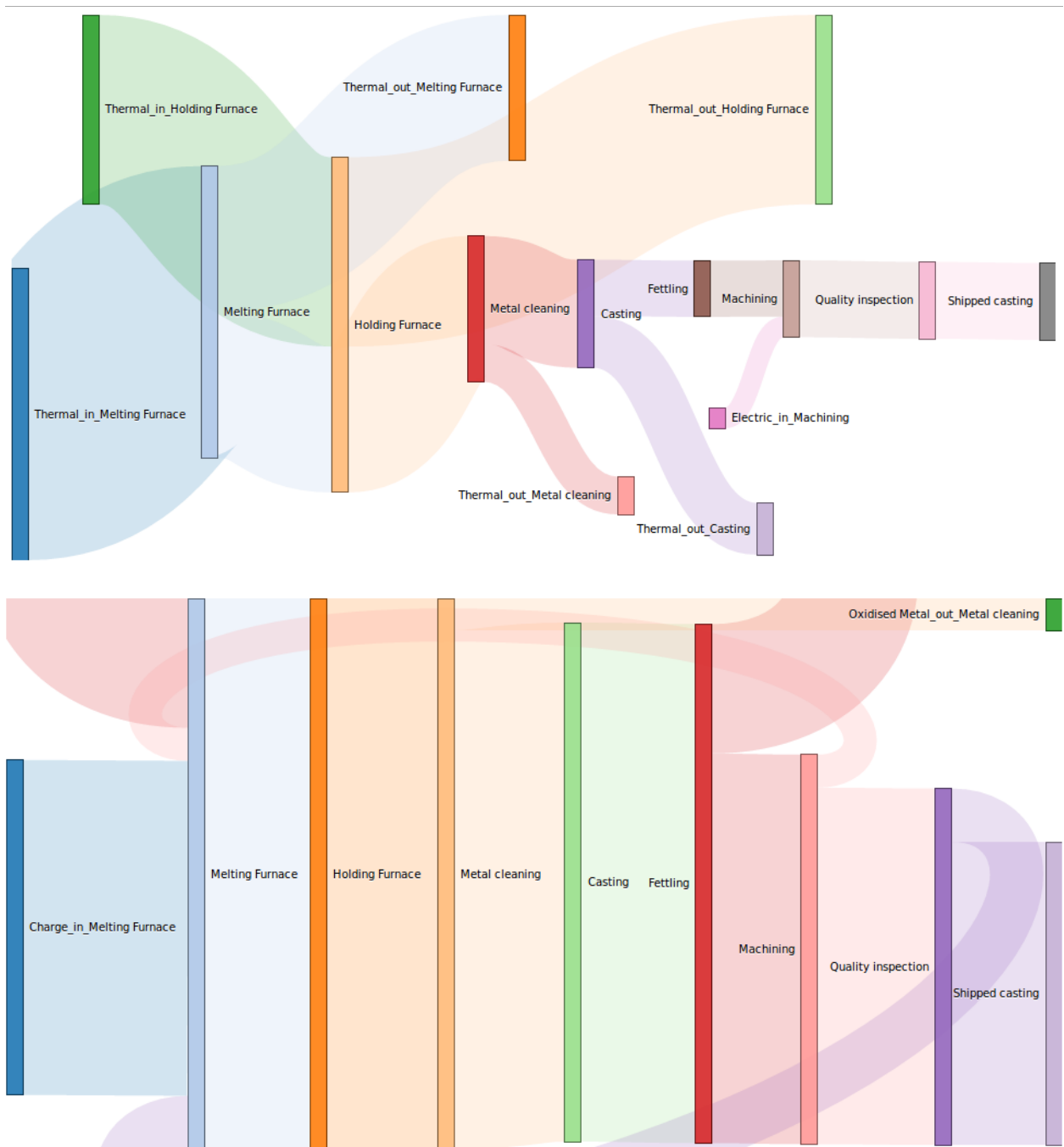
Fig. 11. Example of material (top) and energy (below) flows in Sankey diagrams of a metal casting foundry. The diagrams have been generated by the computer program developed for the “Small is Beautiful” project [42].
