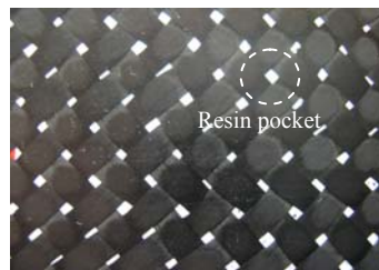
Figure 3.27: Fabric architecture and potential resin rich areas for a single layer braid.
