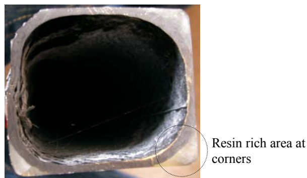
Cross-section (middle beam – after test)
