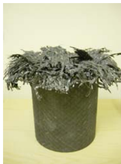
Figure 2.12: A braided tube having a \pm 45^\circ braid angle after axial compression.
