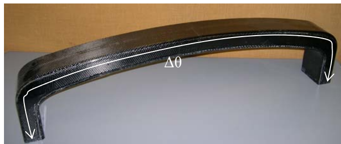
Figure 7.1: Example of a bumper beam with varying braid angle.
