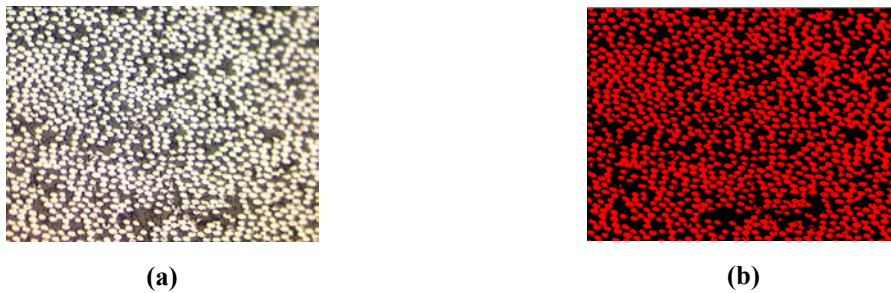
Figure 3.7: Fibre volume fraction determination within a tow from a [\pm 30^\circ] coupon.
