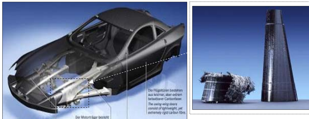
Figure 2.1: SLR crash cones used in frontal impact [37].
