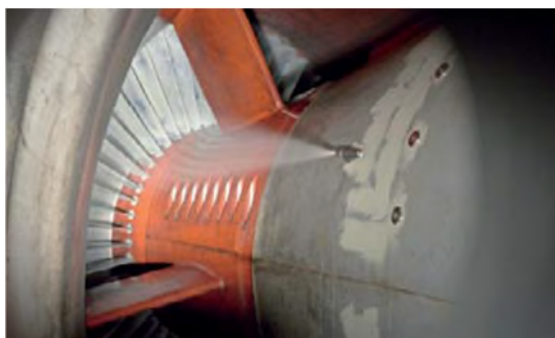
Figure 6 Compressor washing spray injection with nozzle at the plenum [21]
