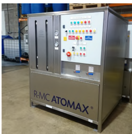
Figure 7 Compressor washing system
