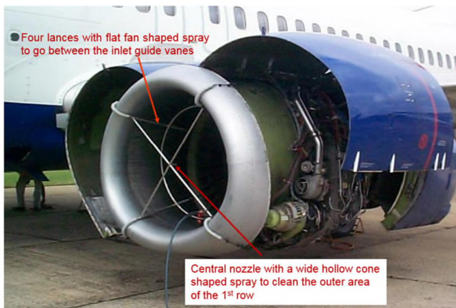
Figure 3 Example of on-wing compressor washing
