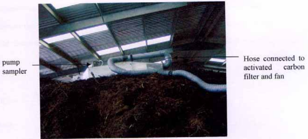
Figure 3.8: Portable wind tunnel located on top of compost pile at Carmarthen Composting.
