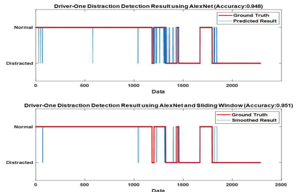
Fig. 12. Driver 1 real-time activity detection using AlexNet and sliding-window.
