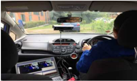
Fig. 2. Experiment setup. The Kinect is mounted on the middle of the front window and data are collected using a laptop.
