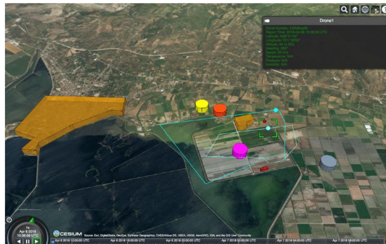
Figure 11. Three drones in VLOS operations and two drones in fully automated BVLOS operations utilizing the DronAssistant.
