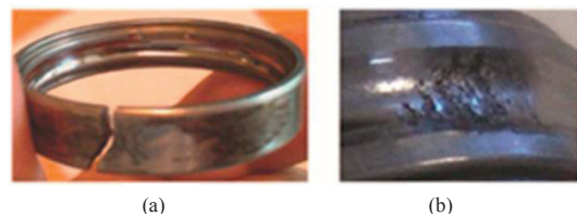
Fig. 2: Bearing (a) external ring failure, and (b) inner ring failure with fracture (Source: [3])
