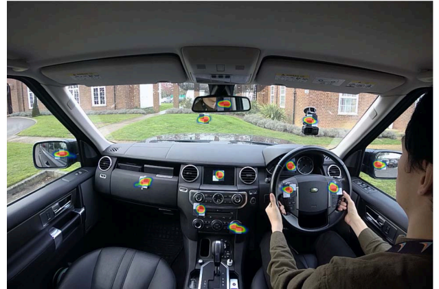
Fig. 6. The accumulated eye gaze mapping for the vehicle experiment.
