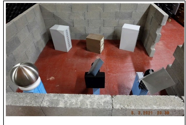
Figure 3-4 , Mock concrete building with targets inside. The metal cabinets to the rear are non-aligned with structure, giving rise to specular flashes and wall-multipath visible in different bistatic geometries.
