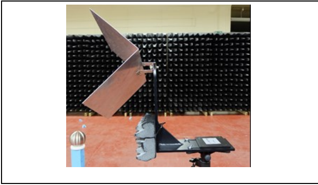
Figure 3-2 , Sphere and dihedral targets. The dihedral was rotated to multiple angles.
