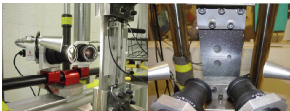
Fig. 8. Stereo DIC camera arrangement and sample on the MTS test frame [34].
