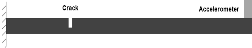
Figure 5: Schematic of cantilever beam with end mass
