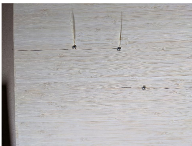
Fig. 6 6 mm Projectile Arrest in Bamboo
