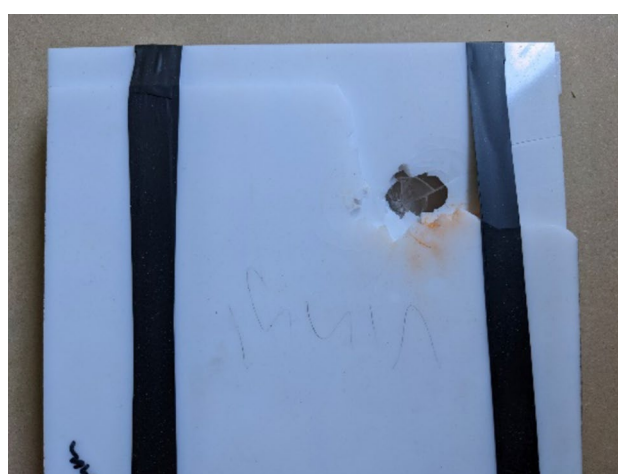
Fig. 7 PVC post impact damage
