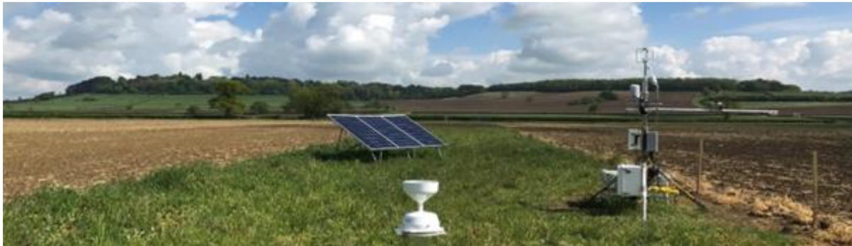
Figure 15. Eddy covariance tower, used to measure GHG emissions.
