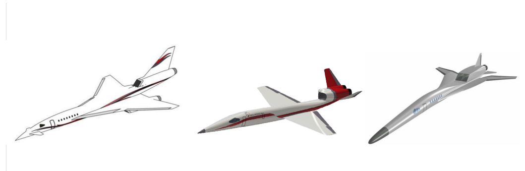
Figure 15. HISAC project concepts for low noise ( left ), long range ( center ) and low boom ( right ). (Source: [144].)
