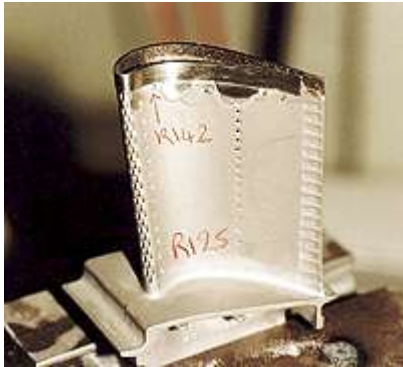
Figure 4. High pressure turbine blade whose tip was formed by the laser cladding process.
